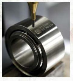
PRYOR MARKING TEC MARKMATE DOT NO 3MM VARIDOT TEX SERIAL NUMBER SERIAL 19/06/201 DATE 19/06/201
